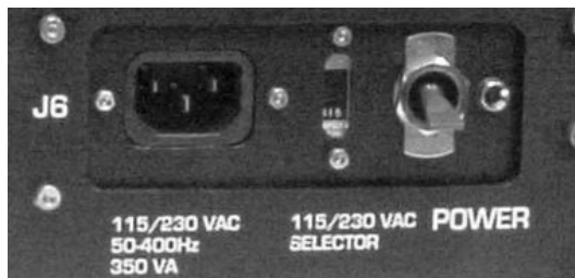
Power Section - SE1420 Controller Back Panel
